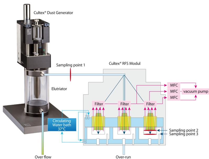
Figure 2: Schematic assembly of the experimental setup for the air-liquid interface exposure
