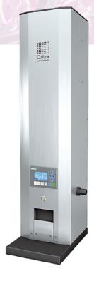
The CULTEX® HyP is a hydraulic press that provides accurate compression of a high variety of dry powders and delivers homogeneous dust cakes for the CULTEX® Dust Generator. The highly encapsulated system is controlled via a control panel and guarantees a secure operational process for the operator under high safety standards as well as precise and highly reproducible results.
