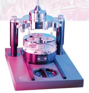
This is a high-end exposure system for the direct exposure of cell culture inserts or Petri dishes. The modular system consists of two main parts, the aerosol-guiding module and the sampling module housing the cell culture inserts, or Petri dishes.
